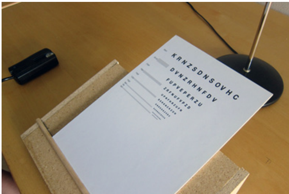
Figure 8. Test of visual acuity. The font is Helvetica CY bold with double spacing between characters. Each line has the same number of characters, and each line includes visually similar characters like R and K or D, C and O. Size of characters from 4 to 36 pt.
