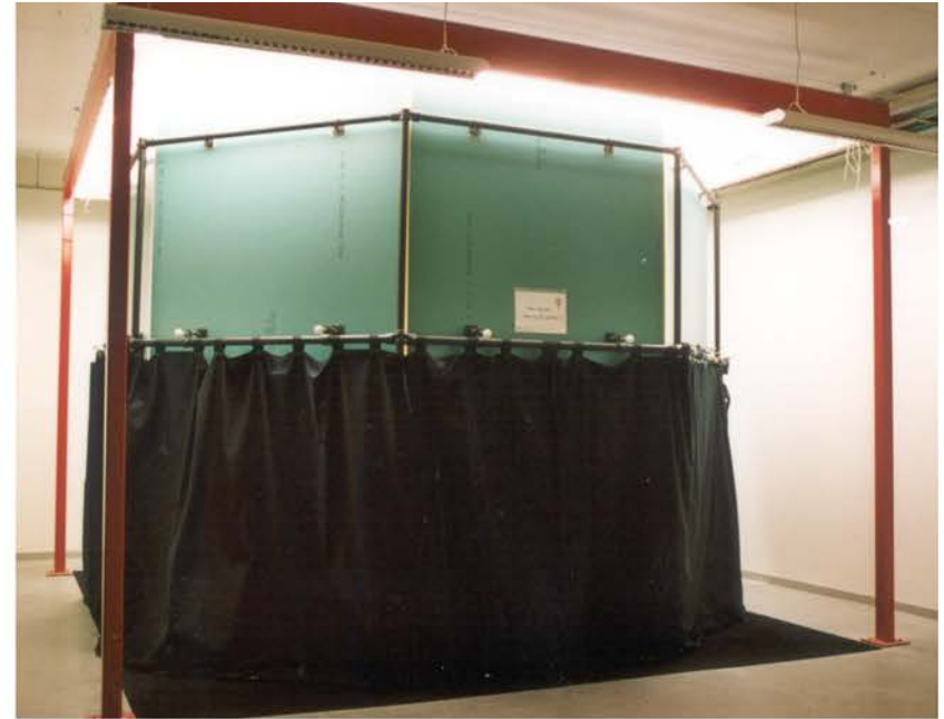
Figure 5. The artificial sky seen from the outside.
